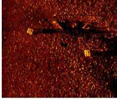
Figure 4. Side-scan sonar image of crab pots on river bottom (Marine Sonic Technology, Ltd.)
